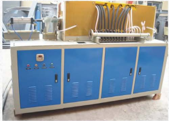
Induction heating cabinet-2
