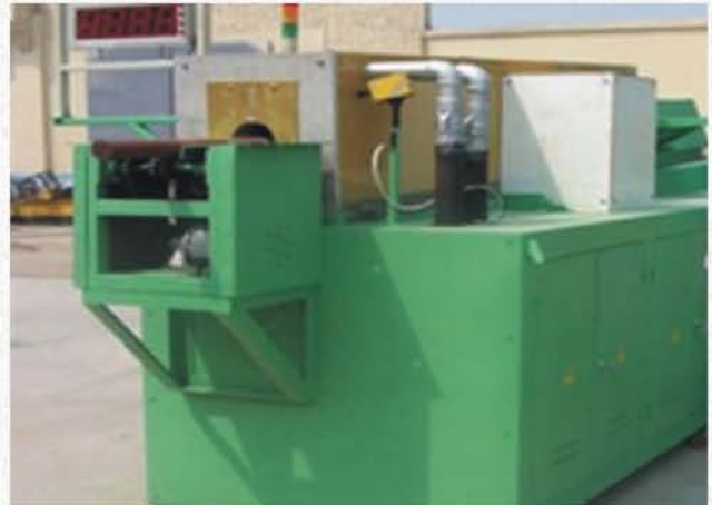
Induction heating cabinet with thermal detector and auto discharge unit
