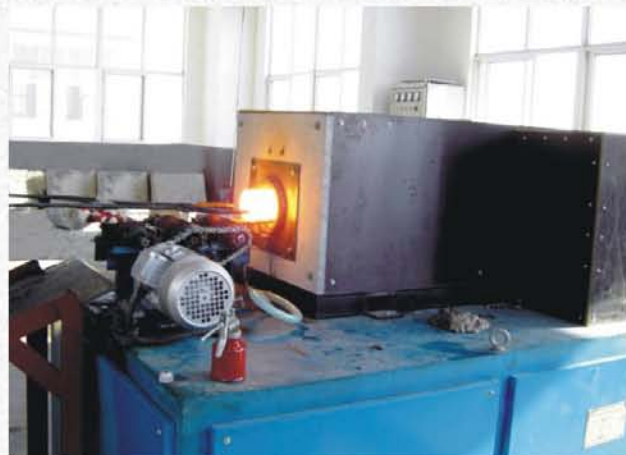
Induction heating cabinet with auto discharge device
