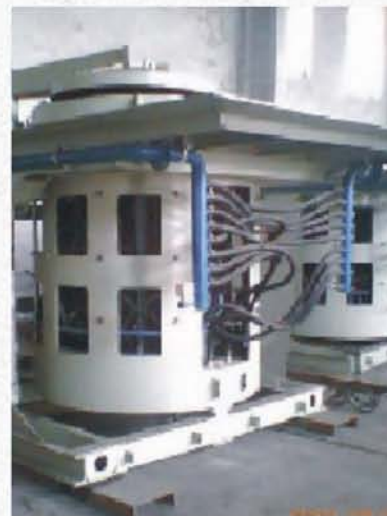
卷筒结构熔炼炉 Drum-type Steel Furnace Body
